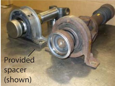
Step 4: Do not forget to include the rectangle spacer block... This is necessary to provide the same bearing height that was used on the OEM design Ford Trucks... the photo has the spacer under the service kit to show how it will provide the same center line height as the original. It must be included when you're ready to weld, balance and install the assembly.
