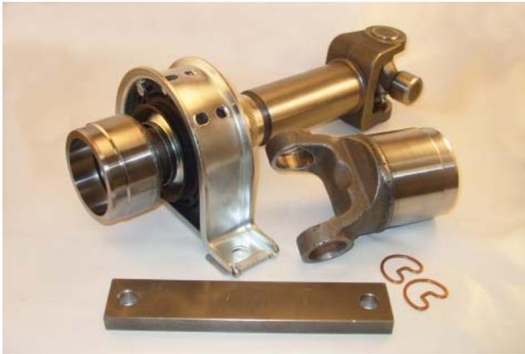
The OEM Ford rear drive shafts have a Non-replaceable center support bearing. With the Rockford Kit you are able to cut the Original assemblies apart at the friction weld and replace the Slip Yoke, Splined Stub and Center Support Bearing... avoiding the additional cost required to build an entirely new assembly.
