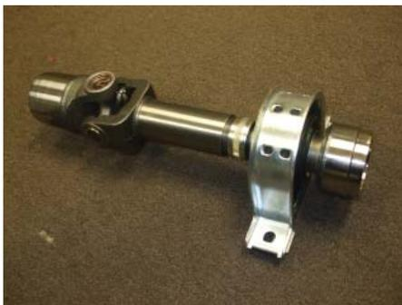
Step 3: The proper way to assemble the Rockford kit is illustrated with the photo shown. The midship stub shaft is pressed into the front OEM tube and welded in place. The weld yoke is pressed into the rear OEM tube and welded.
