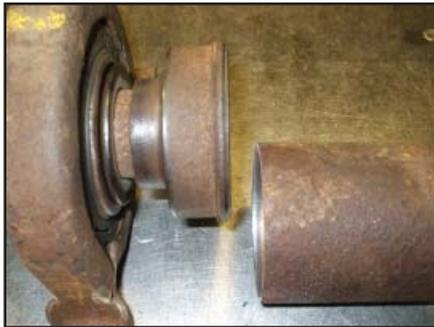
Step 1: Cut the original tube right behind the friction weld on the stub of the center support bearing and then again behind the friction weld of the splined stub and original tubing.
